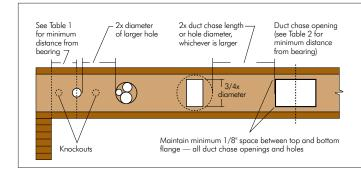
Knockouts are prescored holes provided for the contractor's convenience to install electrical or small plumbing lines. They are 1-1/2 inches in diameter, and are spaced 15 inches on centre along the length of the I-joist. Where possible, it is preferable to use knockouts instead of field-cut holes.
