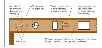
Knockouts are prescored holes provided for the contractor's convenience to install electrical or small plumbing lines. They are 1-1/2 inches in diameter, and are spaced 15 inches on centre along the length of the l-joist. Where possible, it is preferable to use knockouts instead of field-cut holes.
